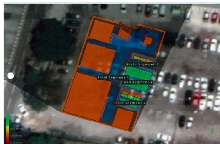
Figure 26 sample roof with solar panel integration produced by a solar PV vendor
